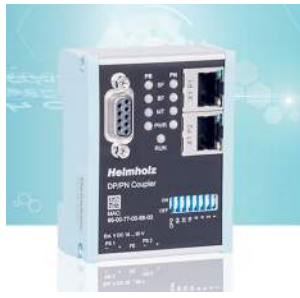
PROFIBUS/PROFINET coupler Connect PROFIBUS and PROFINET networks
