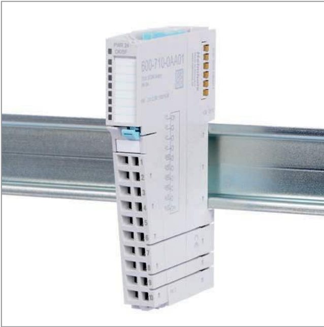
Power and isolation module 24 VDC, 8 A
